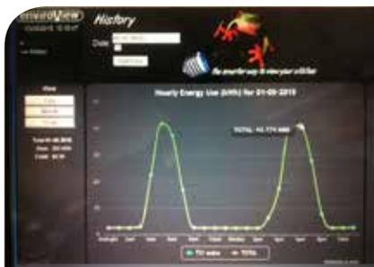
Figure 4 Software output for energy monitoring showing energy use on vat circuit
